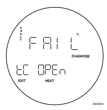
Figure 6-5. Fault 1, Open Thermocouple
